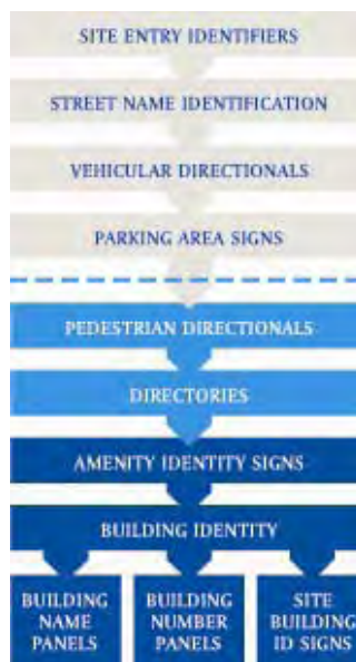
Figure B-8.2 Sign Types Follow a Logical Order and Sequence from the Roadway Entrances to the Final Building Destinations
